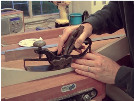
2 Using a good old-fashioned compass plane to get a crisp, accurate edge
