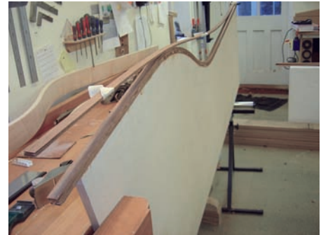
4 The top having been lipped in stages, is now dry and ready for the mitre cut
