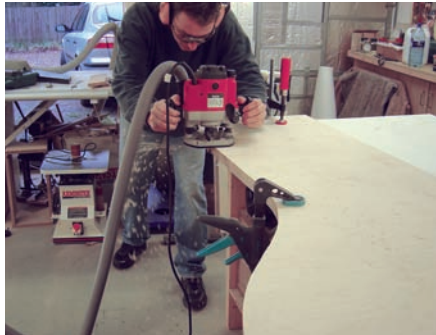
3 A flush trimming bearing guided cutter produced an exact copy of the original
